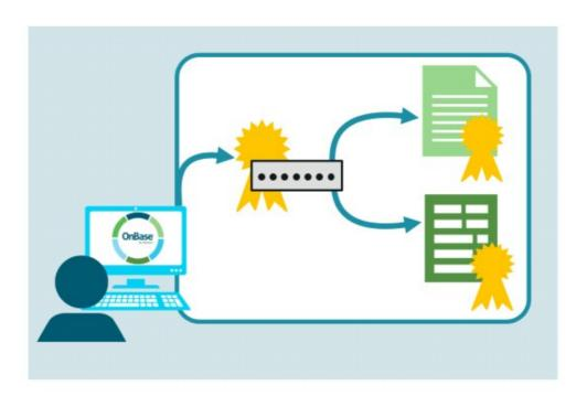
When a user applies a signature to a document through an OnBase client or a Workflow task, Digital Signatures creates a unique value by combining the document data and the digital certificate, and this value is used to validate the signature to ensure the document is unaltered.
