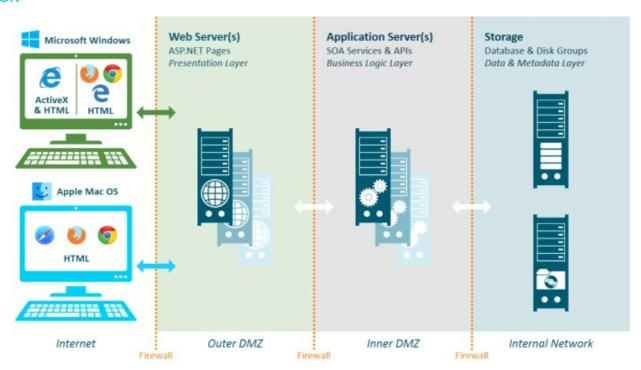
Standard browsers function as secure Web-based clients to the centrally managed OnBase Web Server. The architecture allows the separation of the Web Server and Application Server, providing enhanced performance, scalability, and security options.
